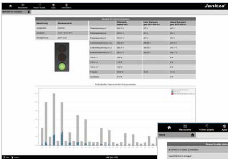
Fig.: IEC 61000-2-4 analysis with traffic-light principle
