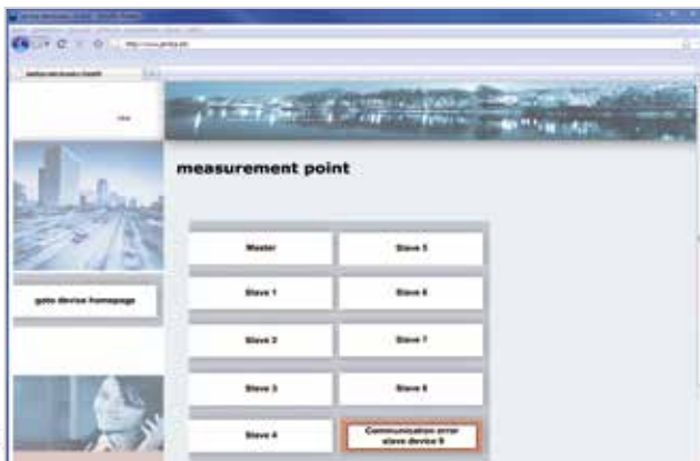
Fig.: Multitouch APP: Slave measurement devices overview on the master device homepage, e.g. up to 31 UMG Modbus slaves can be displayed via a UMG 604-PRO master device
