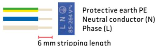
The installation wire up to 1.5 mm<sup>2</sup> can be inserted directly into the spring-loaded terminal. If a stranded wire is used for the installation, push the terminal fully down to insert the stranded wire and only release it once the latter has been positioned correctly.
